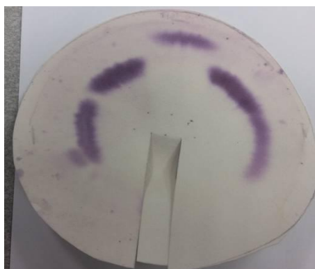
Figure 4 - The procedure and reaction result of Radial (circular) paper layer chromatography
